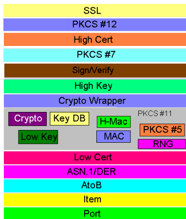
Figure 8: nss layers visualized, from http://www.mozilla.org/projects/security/pki/nss/nss-guidelines.html
